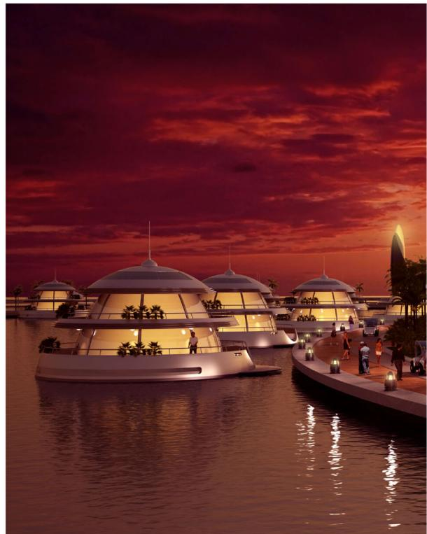
*It is possible to move around the various areas of Amphibious 1000 thanks to the "Trilobis" eco-yachts. These 20 m long vessel is made of aluminium and equipped with a submerged "bulb" for observing the underwater environment: the engine is made of hydrogen-fuelled cells. The links to dry land take the form of small electric vehicles which can move along the piers. At the end of each pier there are lamps marking the park terminals.*
